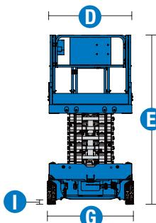
(1) The metric equivalent of working height adds 2 m to platform height. US adds 6 ft to platform height.
